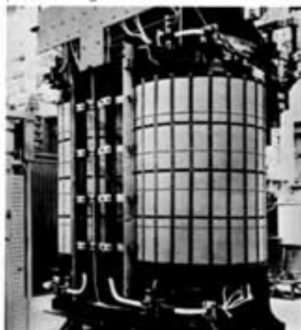
Large power transformer showing Insulam EH lead supports and pressure rings.
