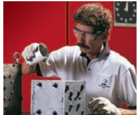
*Cast resin components can be made in our hand-pour shop or in automated pressure gelation, depending on the quantity of parts you require*
